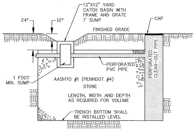
TRENCH SHALL BE LINED WITH PADOT CLASS 1 GEOTEXTILE MATERIAL PER PUBLICATION 408, SECTION 212.3b. ALLOW 1' OVERLAP ACROSS BACKFILL AT TOP OF TRENCH AND ALSO AN OVERLAP OF 1' AT END OF ROLLS.
